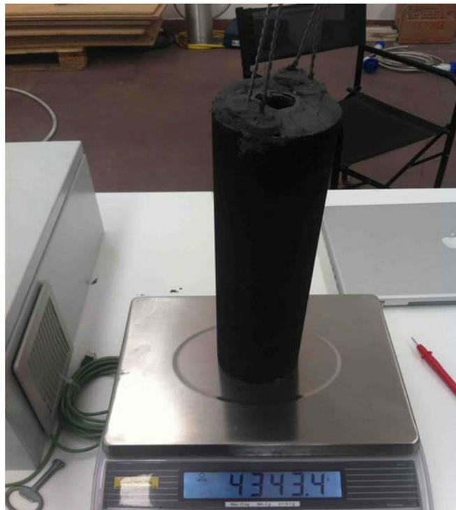
The module is consists of an assembly of four components, plus the active charge (Nickel and catalyzer) and a tablet which acts as a hydrogen reserve. Tablet and charge masses are not known. The module is sealed with Saratoga TE7 1200 1200° smelter-grade putty sealant.
