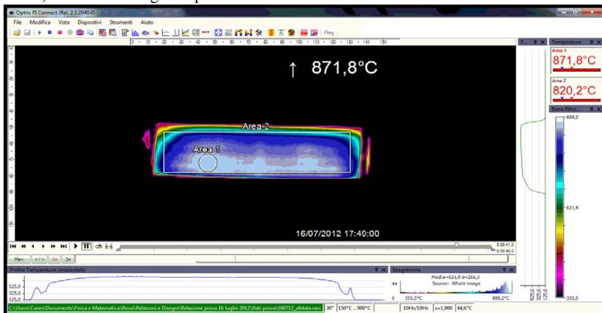
However, frame matrix data indicate that the temperature recorded off the side of the cylinder falls to slightly above 300° C, which is not compatible with average and peak temperatures.
