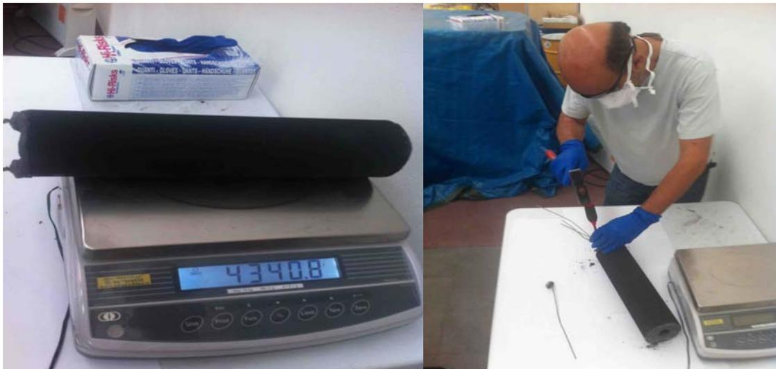
The inner cylinder was weighed first; its weight was seen to have decreased from an original weight of 705.4 g to 702 g. The decrease in weight of 3.4 g is presumably due to the partial loss of coating and to the surface melting of the steel, which appeared rough to the touch.
