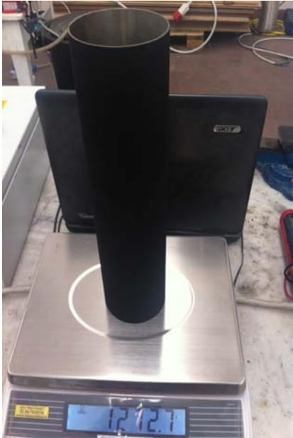
The second component is the inner cylinder, made of the same stainless steel alloy:  $\varnothing$  3.385 cm, weight 705 g, as measured before assembly. The cylinder was subsequently painted on both outer and inner surfaces with black coating, heat resistant up to 1200°.
