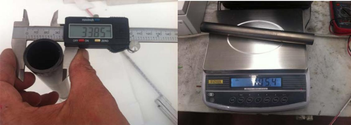
The third component is a set of two 220 V resistors, total weight 2292.8 g; resistance values measured at the start of the test are 11.8 and 12.2  $\Omega$ . In parallel the recorded value was 6  $\Omega$ . Resistors were powered in parallel.
