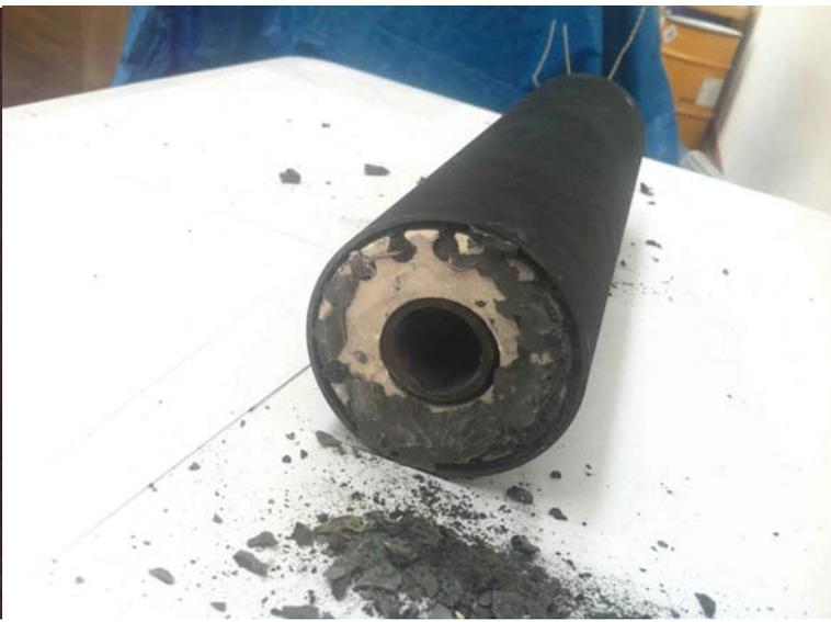
The putty sealant was only partially chiseled away, and was collected on a sheet of paper. The tare weight of the sheet of paper, 4.6 g, was subtracted from the resulting weight of 32.3 g, thus giving a net weight of 27.7 g of putty.
