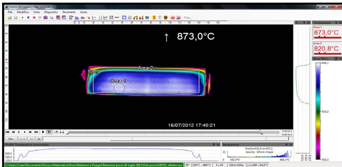
The test was terminated at 5:50 PM in order to keep the data within the infrared camera's range of measurement (150° to 900 C).
