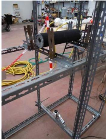
The distance between camera lens and the lower surface of the module is 70 cm.
