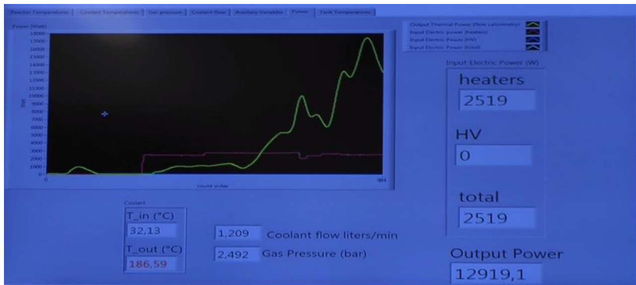
Figure 8 Screenshot of the test performed by DE using Ar and without using the HV excitation
